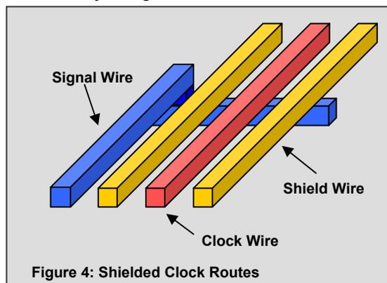
Experimentation using the shielded clock routing technique was done by constraining the clock routes to prefer the third and fourth metal layers, leaving the first and second metal layers
